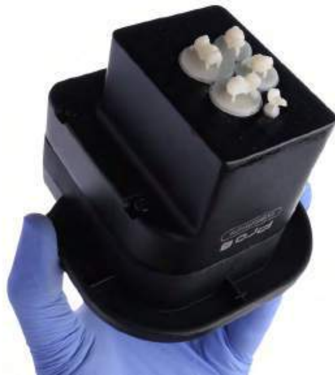
FIG. 8 Final results of the 3D printing phase: the restorations are ready for the next steps.
