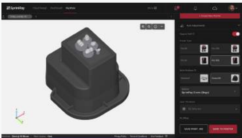
FIG. 5 Design file ready to be sent to the SprintRay Pro 95S 3D Printer. The SprintRay software hub for printing is RayWare.
