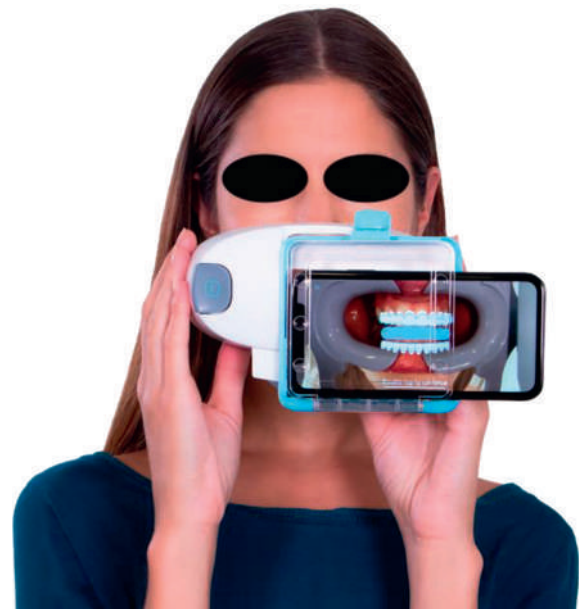
FIGURE 2: Dental Monitoring system. This smartphone-based app allow patients to scan directly their teeth and provide instantaneous feedback of treatment progress to the clinicians and orthodontic office. The patient insert the smartphone into the ScanBox that allows a more predictable scan procedure.
